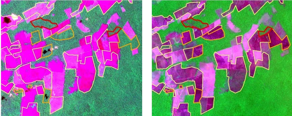
Figure 77: Distribution of 2020 pasture maintenance fires (light yellow), fires after deforestation (orange) and forest fires (red) over Sentinel-2 imagery from 2019 (31<sup>st</sup> July) and 2020 (9<sup>th</sup> October) near the town of Apui in the South of Amazonas State. Image width: ca. 10 km
